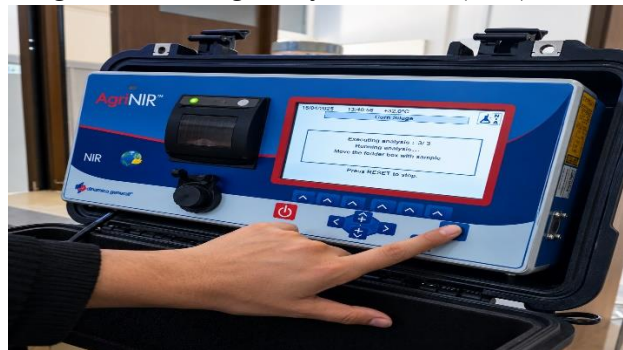
Figure II: Determination of physiological content using a Near-Infrared (NIR) Analyzer
